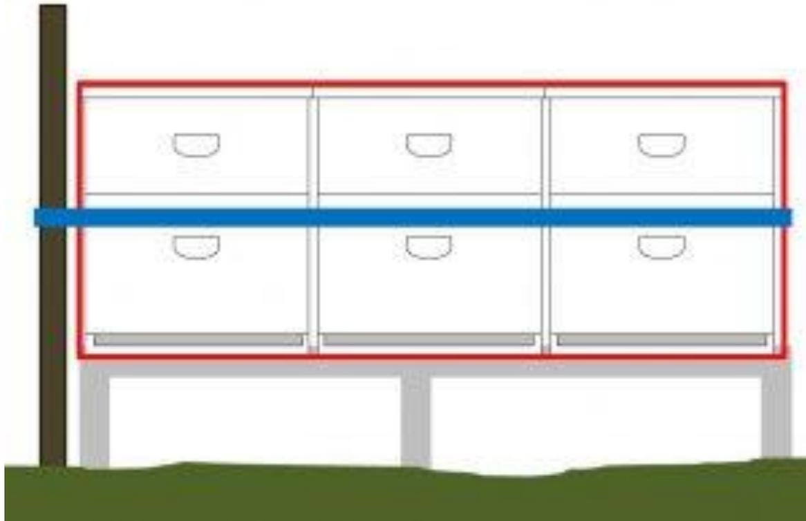
Figure 1: Secure hives. 1) Tighten a ratchet strap vertically around hives [shown in red] to keep the lids secure. 2) Drive a post into the ground and secure hives to it with a horizontally placed ratchet strap [shown in blue].
